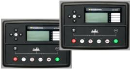
The optional control system for this model is BC 701 (photo), based on the Deep Sea
